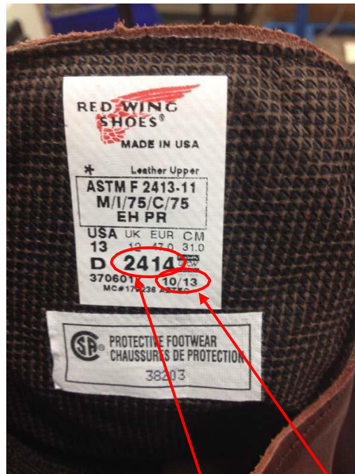
Photo 2: Label inside the boot's tongue Style number Date code
