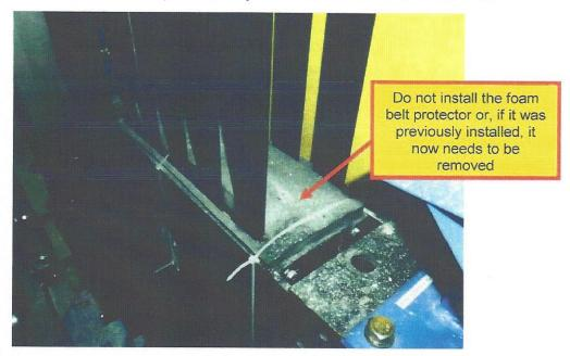
In order to protect the belts and sheave from debris, order and install durable mineral wool that has been approved for this purpose (Florence part # AAA27CJ2).
