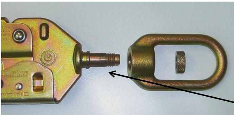
BAD HOOK. STEM OF HOOK BODY WAS NOT SWAGED OVER NUT. THREADED NUT IS CAPABLE OF SPINNING OFF THE STEM.
