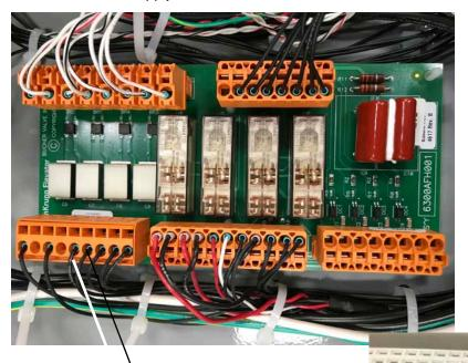
Confirm CON1 Pin  $\hat{\sigma}$  is connected Pin 4 on power supply.
